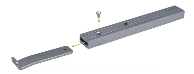
2. Use a 5mm drill bit to open the hole and allow for fitting of the knob
